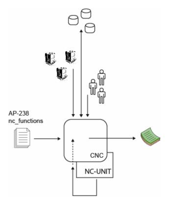
Another important observation for these functions is that "asynchronous events" such as operator log-in/log-out, and machine events are that their essential data is the "event time", so to connect this data with CNC machinig traceability (workingstep/features), it will be needed a complete trace of workingsteo execution time.
