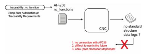
2. NC-Functions standardize the automation process (requirements) and also the data format (structure) of traceability logs. With this approach there are two alternatives.
